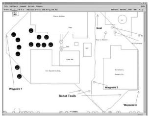
**Figure 6**: Navigation using an internalized plan constructed with only obstacle knowledge guides the robots. As in the previous experiment, each robot proceeds to a waypoint before going to the goal.
