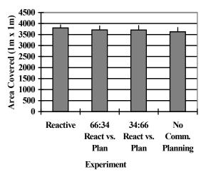
**Figure 10**: Mean Total Area covered per experiment. Using reactive behaviors alone does result in significant improvement in coverage.
