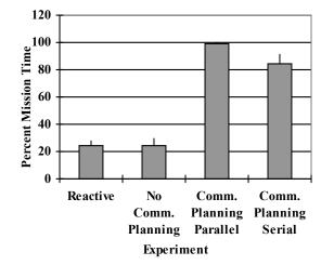
Figure 11: Percent time as a single network per experiment. The use of additional resources in the form of internalized plans results in a drastic improvement in communications.
