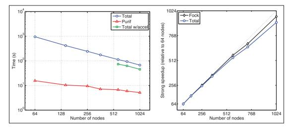
Figure 5. Timings and speedup for one SCF iteration for Ihsg\_80 (9584 basis functions) on Stampede.
