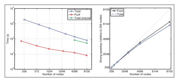
Figure 6. Timings and speedup for one SCF iteration for Ihsg\_180 (27,394 basis functions) on Tianhe-2.
