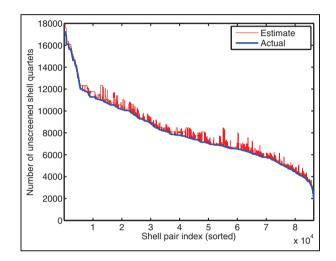
**Figure 2.** Number of shell quartets in each shell pair after screening, sorted by decreasing number of shell quartets. The graph shows that the estimate is a good upper bound on the actual number. The molecular model is the alkane  $C_{24}H_{50}$  with the cc-pVDZ basis set, giving 294 shells and 586 basis functions. The bound would be looser for larger molecules.
