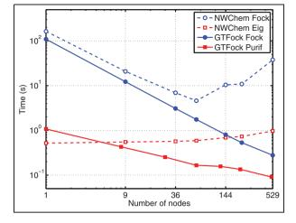
**Figure 1.** Comparison of NWChem to GTFock for 1hsg\_28, a protein-ligand system with 122 atoms and 1159 basis functions. Timings obtained on the Stampede supercomputer (CPU cores only).
