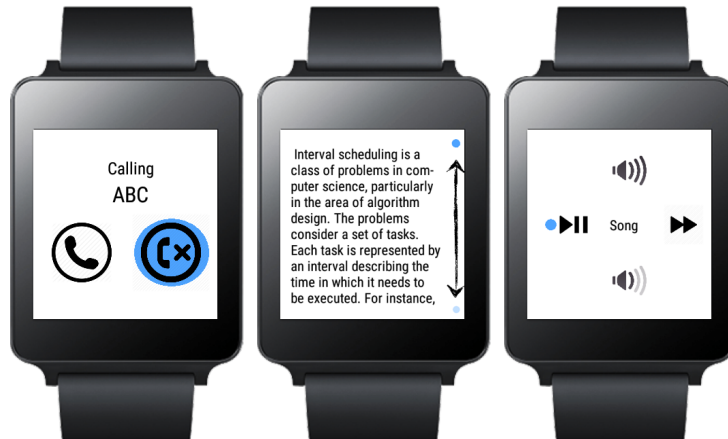
Fig. 16. Figures highlighting three demonstration applications: answering/dismissing a phone call, scrolling through a text view, and controlling a music player.
