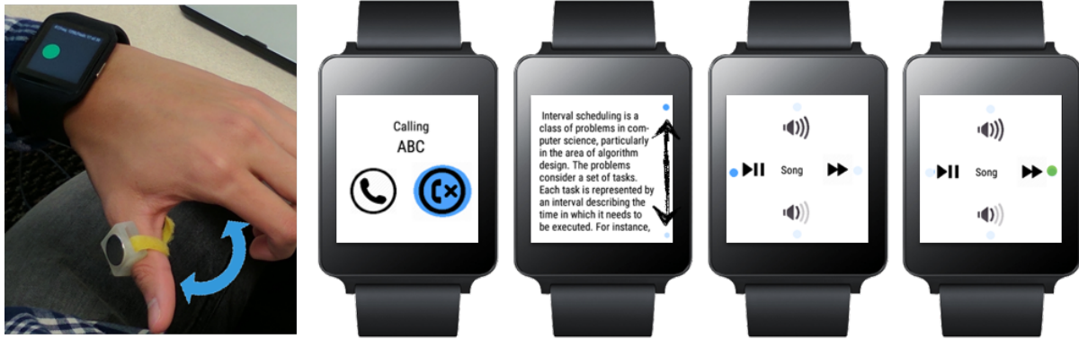
Fig. 1. (A) Synchro is a one-handed interaction technique for smartwatches that uses rhythmic correlation between the user's thumb and binary blinking controls. (B) A demonstration application with a blinking dismiss to voicemail icon (in blue). (C) Blinking targets can be placed in a vertical layout, such as in this reading application. (D) A music player with four possible targets. A wrist flick gesture is used to toggle between pairs of binary targets. (E) The intent to 'sync' is detected when the thumb is repositioned (close to the hand) and icon color changes indicate detection.
