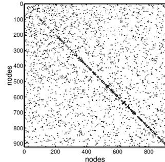
Fig. 4. The connectivity matrix of a topology constructed using  $A'_{\mathcal{H}}$  for  $c=1$ . The strong dependencies are reflected in the concentration along the diagonal. However, there are many points away from the diagonal and the picture appears random.
