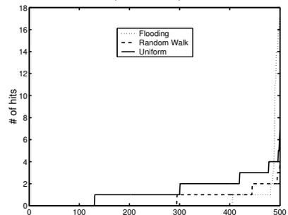
Fig. 3. Performance of searching in A) a network with heavy-tailed statistics, and B) in a real topology. The small TTL in the real topology is due to the fact that using a larger TTL would have resulted in reaching with flooding almost half of the nodes, which is unrealistic.
