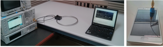
Fig. 9. Measurement setup for laptop or desktop (left) and measurement setup for cell-phone (right).
