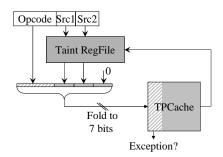
Figure 3. Taint propagation in FlexiTaint
