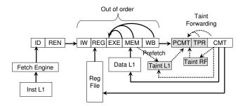
Figure 2. Processor pipeline with FlexiTaint
