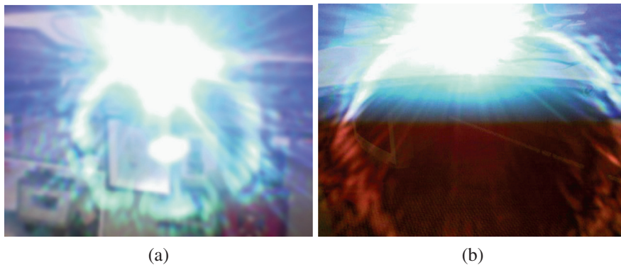
41 Fig. 5 Images taken from a camera hit by localized light beam emitted by our camera neutralizer. 42 The picture on the left shows a localized light beam generated using a single color. The picture on 43 the right shows a localized light beam generated using color patterns that do not allow the cameras 44 to adjust to the light source (notice the scan line)
