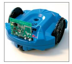
Figure 1. A Parallax Scribbler robot with an Institute for Personal Robots in Education add-on board.
