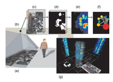
Fig. 1. Viz-A-Vis overview: capture and visualize activity. (a) Place of interest, (b) overhead camera, (c) image sequence, (d) motion sequence, (e) spatial and temporal aggregation, (f) semantic aggregation, and (g) visualization of activity.
