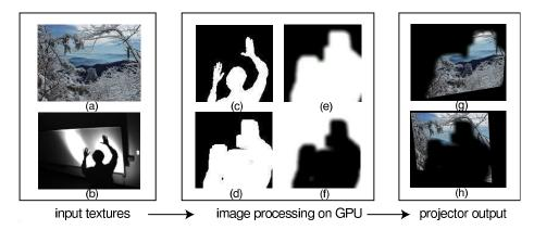
**Figure 21:** *GPU-centric architecture:* (a) display texture (b) IR camera frame (c) occluder mask texture (d) dilated mask to tolerate inter-frame occluder movement (e) blurred mask for projector 1 blending (f) blurred mask for projector 2 blending (g) keystone-corrected projector 1 output (h) keystone-corrected projector 2 output.
