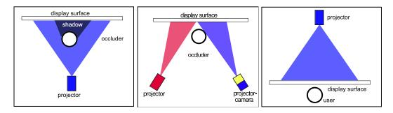
Figure 1: left to right: Front Projection, Virtual Rear Projection, Rear Projection
