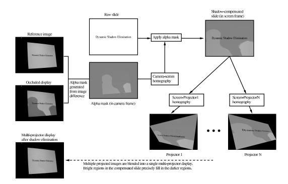
**Figure 13:** This diagram summarizes the occlusion detection and shadow elimination algorithms. The images in the left column were taken by the system camera during operation. The two penumbral occlusions caused by the person blocking both projectors are identified and corrected to create a shadow-free display (bottom left). See text for details.
