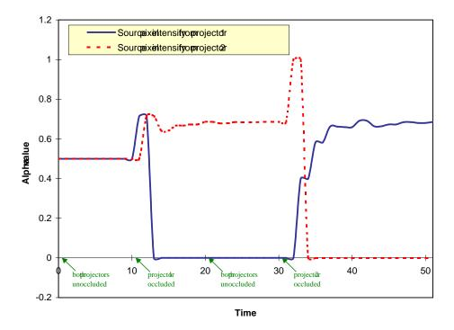
**Figure 16:** Synthetic example of transitions in projector source pixel intensities. This graph shows the intensity transition of two corresponding projector source pixels over time, subject to four events of occlusions and deocclusions. Note the hysteresis effect in which the source pixels are not boosted or blanked until new occlusion events occur.
