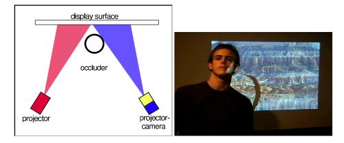
**Figure 17:** *Left:* Switching VRP. *Right:* Shadows are eliminated and blinding light is suppressed with a moving user. The gap in the display caused as the user moves into the scene will be corrected in the next iteration.
