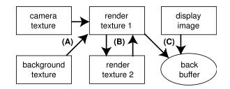
**Figure 20:** *Pixel Shader Pipeline:* Boxes represent textures and arrows denote texture sampling operations used in pixel shaders. (a) Background subtraction shader stores result in render texture 1 (b) Render textures 1 and 2 are used as sampling buffers for dilation and blurring operations, each of which require 2 independent shaders (c) the final occluder mask is composited with a display texture and rendered into the back buffer for display.
