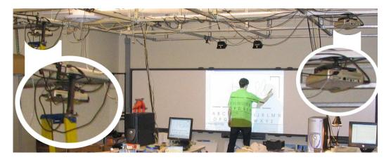
**Figure 30:** A view showing the two projectors (far left above ladder and far right), two IR lights (black, above the user's head), and the SmartBoard. The system is using PVRP in this photograph, and graphics are projected on the users back.
