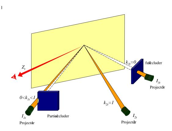
**Figure 14:** Photometric framework. This diagram illustrates equation (2), in which the observed display intensity  $Z_t$  is related to the combination of projector source pixels  $I_{jt}$  and the corresponding visibility ratios  $k_{jt}$ . The visibility ratios vary accordingly with non-occlusion, partial and full occlusion.
