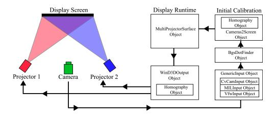
Figure 29: Architecture diagram of the PROCAMS toolkit showing data flow for calibration and use.
