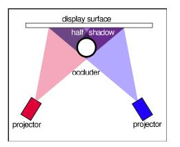
(b) Warped Front Projection
