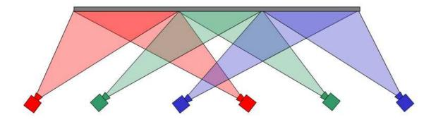
**Figure 10:** Projector locations and beam-paths for a 17.5ft (5.3m) wide electronic whiteboard using passive virtual rear projection. Users find it extremely difficult to avoid standing within projection beams.
