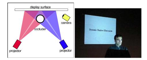
Figure 12: *Left*: Shadow Elimination. *Right*: Penumbral shadows are eliminated but the blinding light remains.
