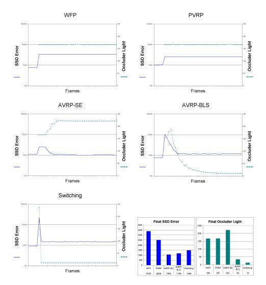
**Figure 22: Top Left:** Warped Front Projection **Top Right:** Passive Virtual Rear Projection **Middle Left:** Active Virtual Rear Projection - Shadow Elimination **Middle Right:** Active Virtual Rear Projection - Blinding Light Suppression **Bottom Left:** Switching Virtual Rear Projection **Bottom Right:** Final SSD and Occluder Light Measures
