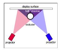
Figure 3: Passive Virtual Rear Projection
