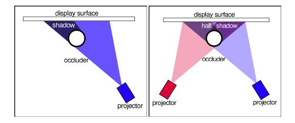
**Figure 23: left:** A Warped Front Projection (WFP) display. The enhanced keystone correction allows more freedom in projector placement. **right:** A redundantly illuminated display (Passive Virtual Rear Projection) uses two or more projectors to increase brightness and provide robustness in the face of occlusions and shadows.
