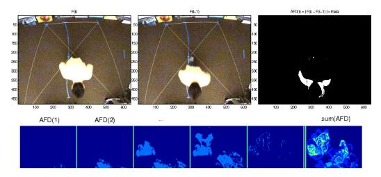
**Figure 36:** Visual explanation of the adjacent frame differencing method. The difference between temporally adjacent frames (*top right*) is summed over time to aggregate user activity.
