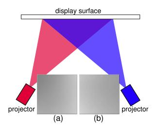
**Figure 19:** *Luminance Attenuation Maps (LAMs):* (a) LAM for projector positioned to the left of projection surface (b) LAM for projector positioned to the right of the projection surface. Note that the dark regions of each LAM correspond with the shortest projection distance to the display surface.
