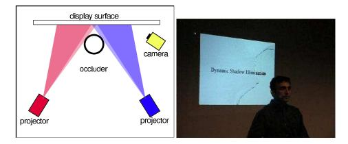
Figure 15: *Left:* Shadow Elimination with Blinding Light Suppression. *Right:* Light is kept off of the occluders face.
