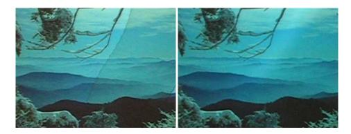
Figure 18: Boundary between regions of varying projector ownership. *Left:* before seam blending. *Right:* after seam blending.
