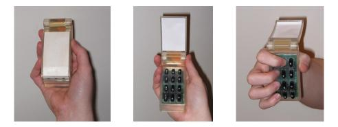
Fig. 4. A mobile phone design which incorporates chording capabilities.
