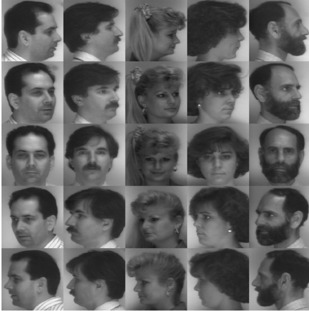
Figure 2: Some of the images used to test accuracy at face recognition despite wide variations in head orientation. Average recognition accuracy was 92%, the orientation error had a standard deviation of 15^\circ .
