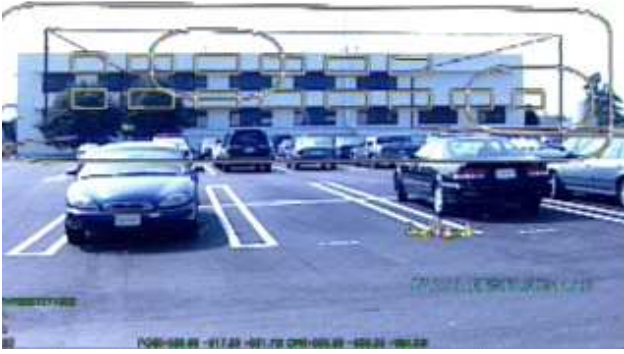
Fig. 1. An example of the use of registration error estimation. The system highlights a building and two of its windows by outlining the areas of the screen the objects could occupy. Each outline was created by growing the convex hull based on an estimate of the registration error. The simple, misregistered computer model of the building is shown for clarity. While the model is not registered with the world, the intended objects fall within the highlighted areas of the screen.
