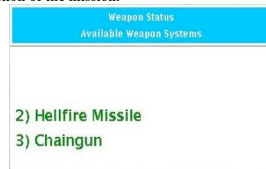
Figure 3. As weapon systems become deactivated, this operator display is updated to show the robot's current capabilities.
