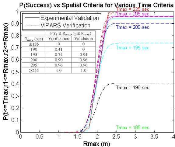
Fig. 13: Verification & Validation of Spatial Criterion at various  $T_{\max}$
