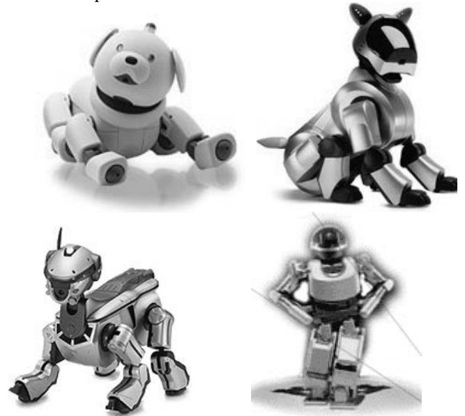
Figure 1. Sony's Entertainment Robots (Top and Lower Left) AIBO Variants (Bottom Right) SDR
