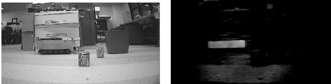
Figure 17: A robot’s-eye view of a laboratory scene including another green robot, two red soda cans and a blue wastebasket. The image on the right shows the image after processing to highlight green pixels. Notice how well the robot stands out.
