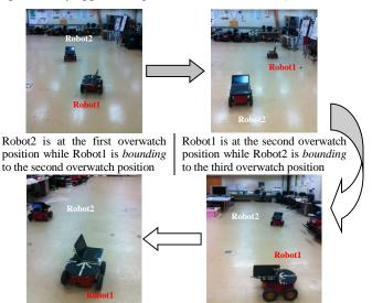
Robot1 is at its goal location while Robot2 is *bounding* to its goal location Robot2 is near the third overwatch position; Robot1 is about turn 90 degrees counterlockwise and bound to its goal location
