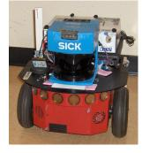
Fig 3. Robots used in the robotic discovery process. (left) B21R robot used with overhead microphone array, and SICK laser mounted in the base. (top) Pioneer-2dxe with microphone array mounted in the rear.
