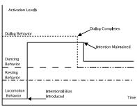
Fig. 9 An idealized graph of activation values for four behaviors demonstrating how intentional bias does not necessarily override existing behavioral expression. In this case the bias is not great enough to make the locomotion behavior run. The bias remains, however, and when the robot finishes conversing with a user, the bias to the locomotion behavior now allows it to run.
