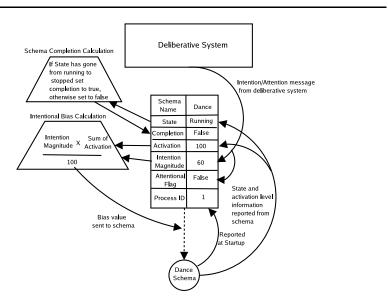
Fig. 7 Dataflow in the intentional bus. Arrows show origin and destination of the data. Trapezoids show computations internal to the intentional bus.
