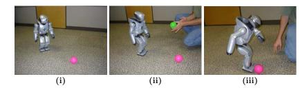
Fig. 19 Depiction of high intention soccer plan. i) QRIO approaches the ball ii) The operator tries to distract QRIO with the green ball (the releasing mechanism for the greet behavior) iii) QRIO kicks the ball and completes the plan.
