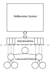
Fig. 5 Overview of the interaction between the deliberative system, intentional bus, and lower level reactive behavior
