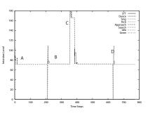
Fig. 20 Activation levels trace during the execution of a low intentional magnitude plan: A) Search behavior is active. B) Approach behavior becomes active. C) Releasing mechanism for greet behavior is found and its activation is increased. D) Intentional bus maintains appropriate intention levels but intentional magnitude is low enough to allow other behaviors to execute. E) Greeting behavior finishes and approach behavior becomes active again. F) Kick behavior becomes active.
