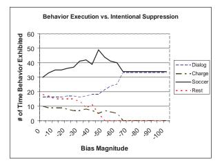
Fig. 16 Behavior exhibited as a function of the amount of intentional bias on the charge and rest behaviors. Demonstrates how intentional bias can provide variable amounts of behavioral suppression.
