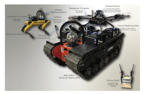
Figure 2: Team CSIRO Data61's robot platforms deployed during the final event.
