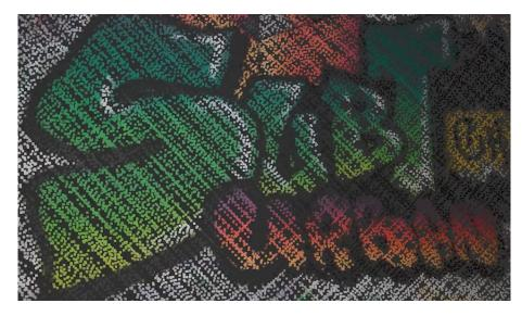
Figure 26: The raw coloured point cloud showing a mural in the circuit, calculated online by Team CSIRO Data61's Bluey platform during the Final Event.
