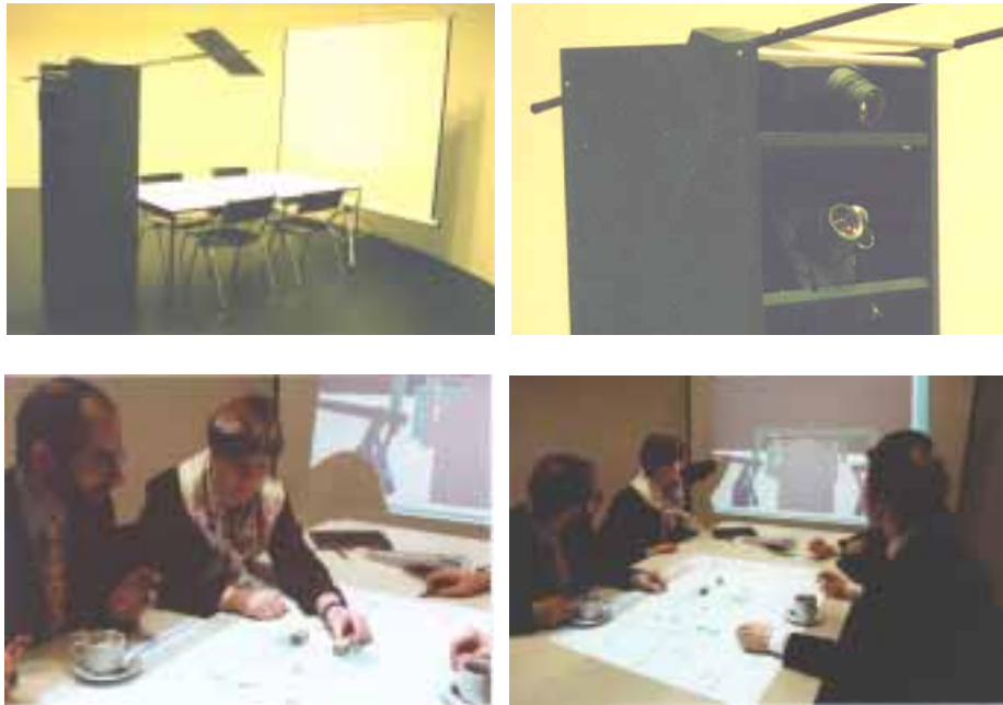
Fig. 1. BUILD-IT consists of a rack, mirror, table, chairs and a screen (top left). In addition to a high-end personal computer (PC), the rack contains two beamers, a video camera and a light-source (top right). The system offers a horizontal plan view for combined action and perception (bottom left), and a vertical side view with a perspective of the situation (bottom right).
