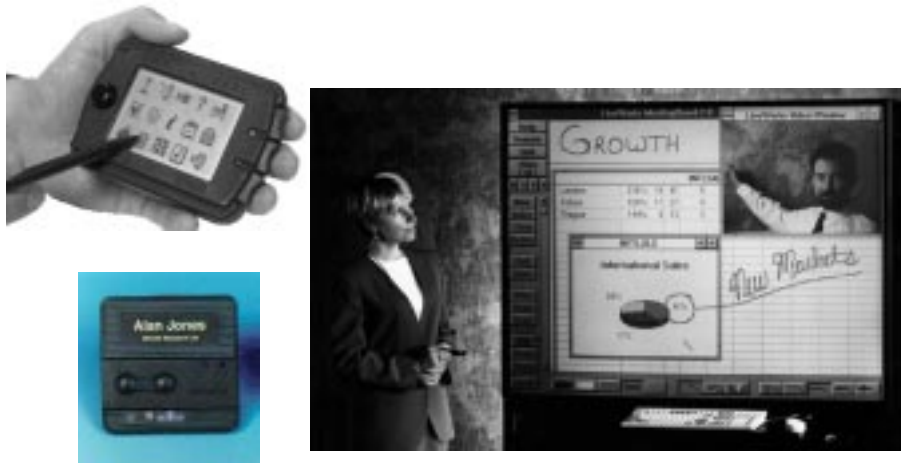
Figure 1: Weiser (1991) described ubicomp devices of different size scales including the handheld PARCTab, the wearable active badge and the whiteboard sized Liveboard.
