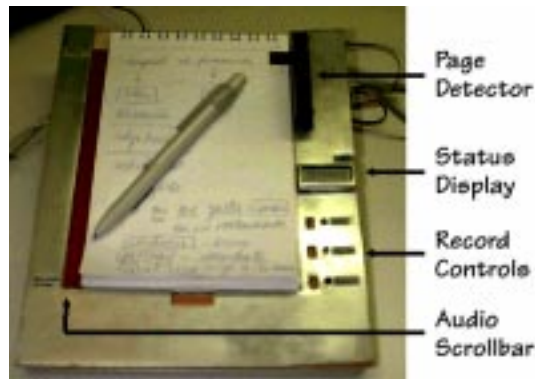
Figure 3: Stifelman's Audio Notebook (1996, 1997) is a good example of implicit natural input—the freehand notes act as indices into the captured audio.
