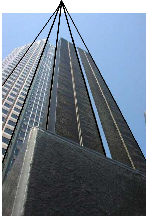
Figure 4: Projections of parallel (here: vertical) lines intersect at one point.
