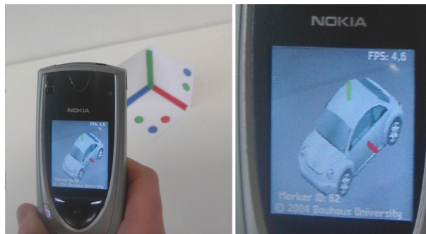
Figure 2: Video see-through example on a consumer cell-phone.
