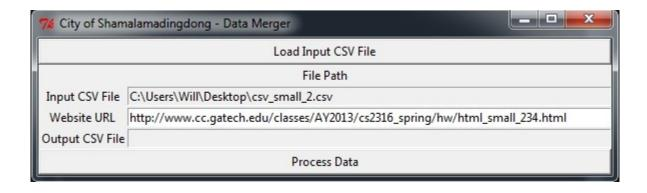
If instead the loadCSVfile method returned a None (indicating that the file was invalid), you should pop up an error dialog message to the user, and leave the input csv file entry blank and the Process Data button disabled.
