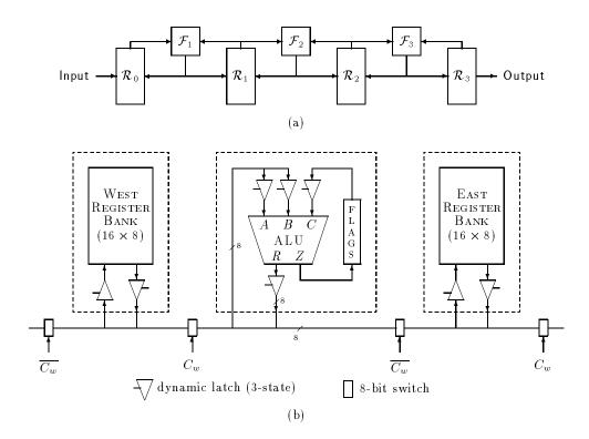
Figure 2: Abstract linear SSRA processor array (a) and the B-SYS architecture (b).
