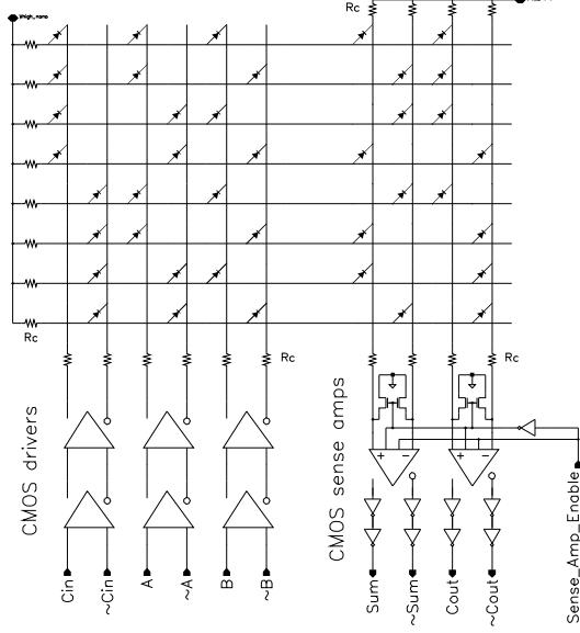
Fig. 5. The system we consider involves CMOS level shifters to drive the nano crossbar and CMOS sense amplifiers to restore the crossbar output to CMOS voltage levels.
