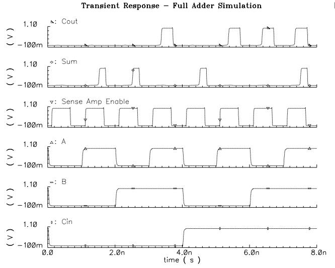
Fig. 7. Simulation waveforms for the nano crossbar and peripheral CMOS show the full-adder crossbar functioning correctly.
