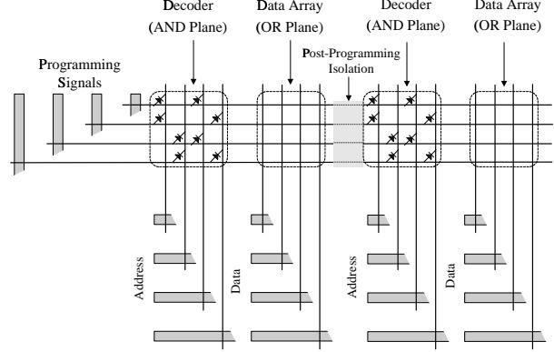
Fig. 3. A platform for logic and memory can be assembled by combining a number of diagonal interface structures.
