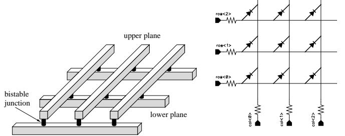
Fig. 1. A typical nanoscale crossbar structure consists of two planes of crossed nanowires with bistable devices at the junctions.
