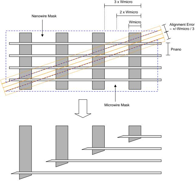
Fig. 2. Pitch reduction can be achieved by employing an interface scheme that relies on alignment accuracy.
