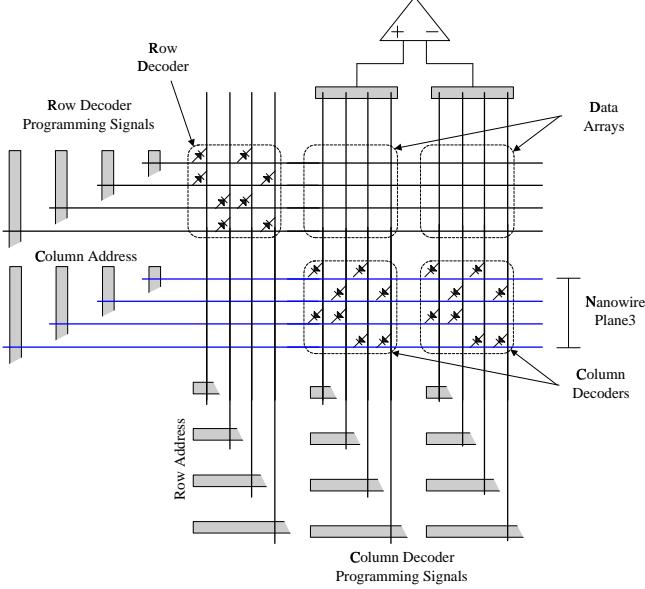
Fig. 8. The addition of a third plane of nanowires allows a column decoder to be included in the nano crossbar structure.
