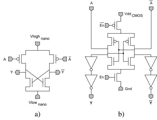
Fig. 6. We use standard CMOS circuits for the CMOS interface, a) level shifters driving the nano crossbar inputs, b) cross-coupled inverter latches to sense the outputs.
