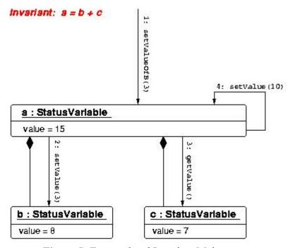
Figure 5: Encapsulated Invariant Maintenance
