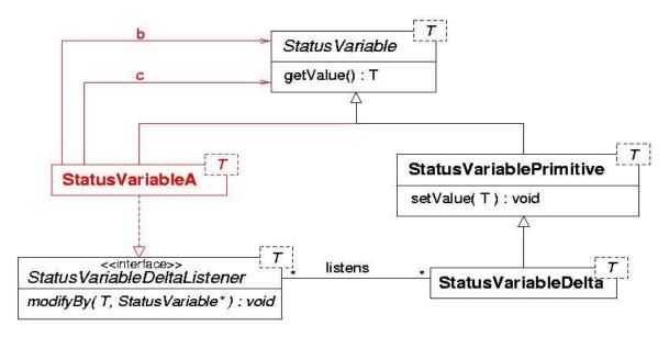
Figure 10: Implementation of Distributed Invariant Maintenance
