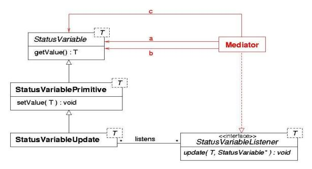
Figure 9: Implementation of Mediated Invariant Maintenance
