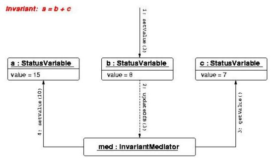
Figure 6: Mediated Invariant Maintenance
