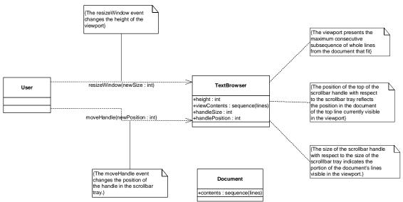
**Explanation:** The diagram contains three actors: the **TextBrowser** in the center, the **User** on the left, and the **Document** in the bottom center. The **TextBrowser** is the as-
