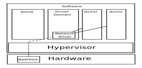
Figure 1: Xen Separate Driver Domain.
