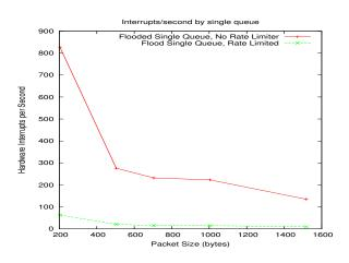
Figure 8: Reduction in Hardware Interrupts to CPU
