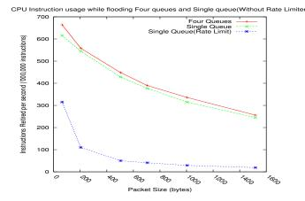
Figure 10: Instructions per second while flooding
