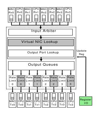
Figure 4: Pipeline for NetFPGA implementation.
