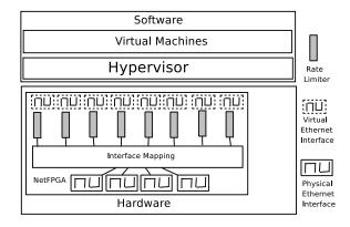
Figure 3: Virtualized network interface card with rate limiters.
