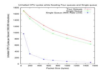
Figure 9: Unhalted CPU Cycles per second while flooding.
