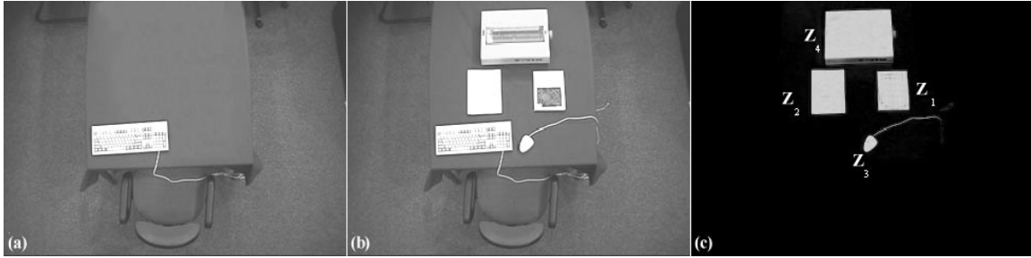
Figure 5.7: (a) Initial background snapshot of scene includes known articles: chair and keyboard. (b) Background after book, notebook, mouse, and printer articles are introduced. (c) Background subtraction reveals newly introduced articles.
