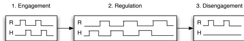
A contingency detector can tell a robot whether to engage or disengage a person (stages 1 and 3). After engaging, the dyad performs turn-taking to regulate interaction timing (stage 2).
