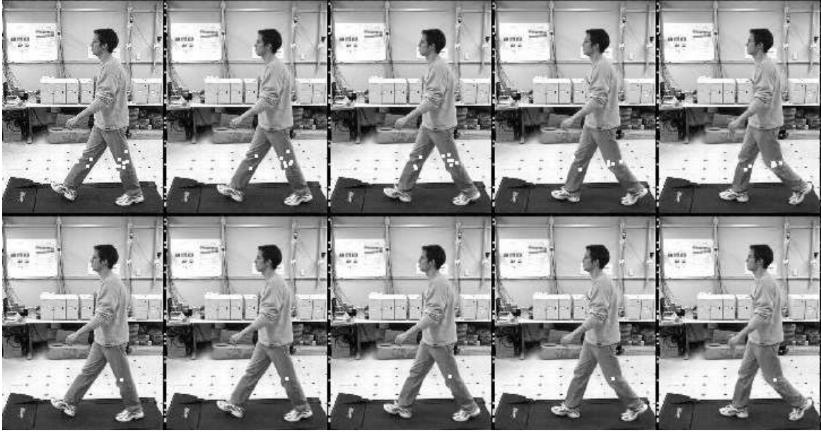
Figure 3. Hidden Markov Model is used to handle the mismatch between left and right limbs. Images in the first row contain the matches for left knee after eliminating noises. In the second row images HMM is used to find the actual position of the joint.
