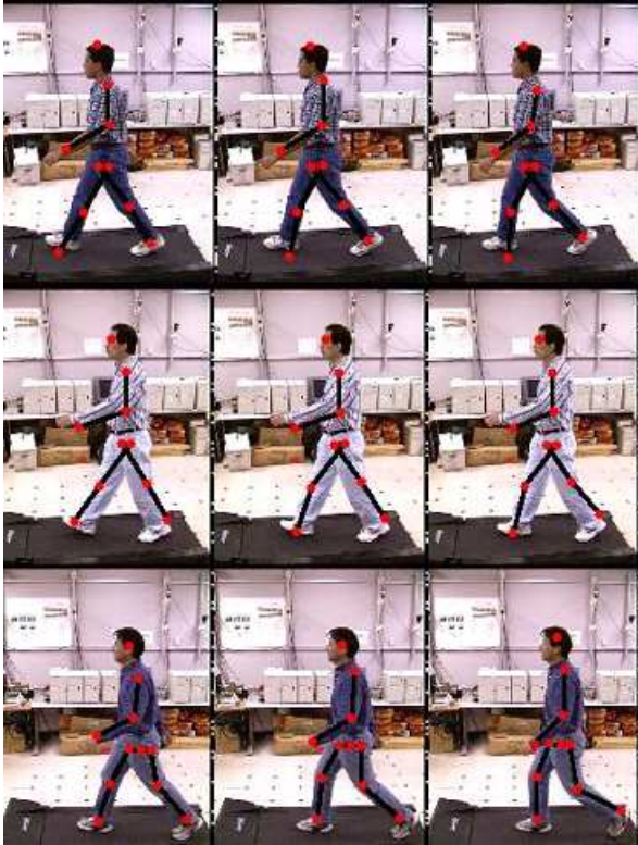
Figure 4. Results. Joint positions of the left shoulder, left knee, left hand and the joints on legs are shown.
