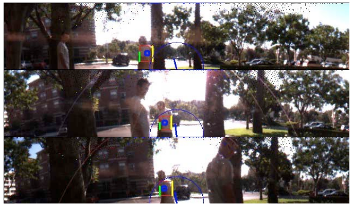
Fig. 6. Output from the omniscam during tracking among trees: the robot is following the person in the middle (top frame - small circle indicates target position estimate), while another person (from the left) is crossing the path between the robot and the first person
