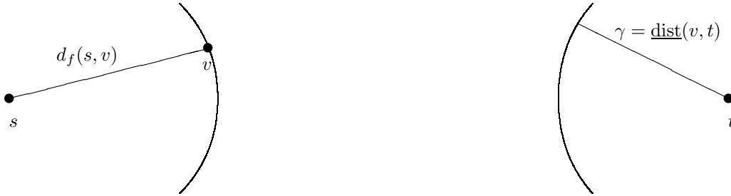
Figure 1: Bidirectional bound algorithm. Assume v is about to be scanned in the forward direction, has not yet been scanned in the reverse direction, and that the smallest distance label of a vertex not yet scanned in the reverse direction is \gamma . Then v can be pruned if \bar{r}(v) < d_f(v) and \bar{r}(v) < \gamma .
