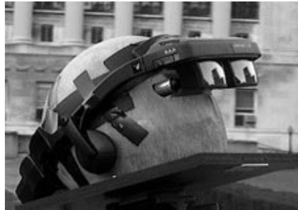
Figure 9. The dummy head used to capture images through our headworn display. A camera in the right eye socket captures what a user wearing the display would see.
