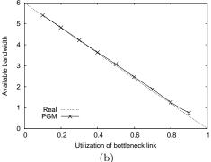
Figure 2: Estimated available bandwidth for a two-hop path with (a)  $C_1$ =6Mbps and  $C_2$ =10Mbps, and (b)  $C_1$ =10Mbps and  $C_2$ =6Mbps. The cross traffic follows the path persistent model.
