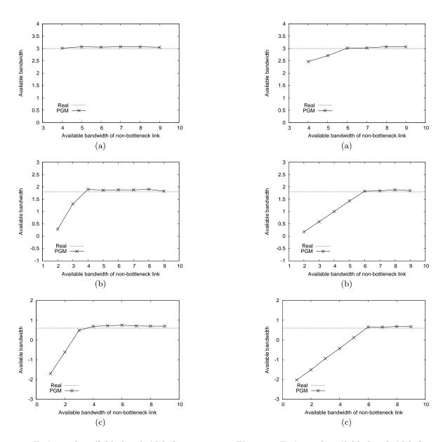
Figure 3: Estimated available bandwidth for a two-hop path with  $C_1$ =6Mbps and  $C_2$ =10Mbps. The available bandwidth  $A_1$  of the bottleneck link is: (a) 3Mbps (b) 1.8Mbps and (c) 0.6Mbps. The cross traffic follows the one-hop persistent model.
