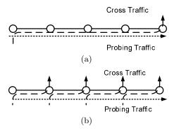
Figure 1: Path persistent (a') and one-hop persistent (b') cross traffic.
