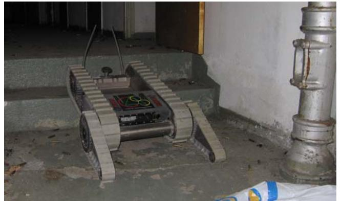
Fig. 1 The Packbot going down stairs while checking out the basement of a residential building block.
