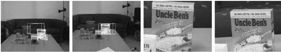
Fig. 5. The first two images show a target region before and after a saccade (the rectangles show the foveal regions within the left peripheral camera image) and the foveal camera images after executing a saccade are shown in the last two images.
