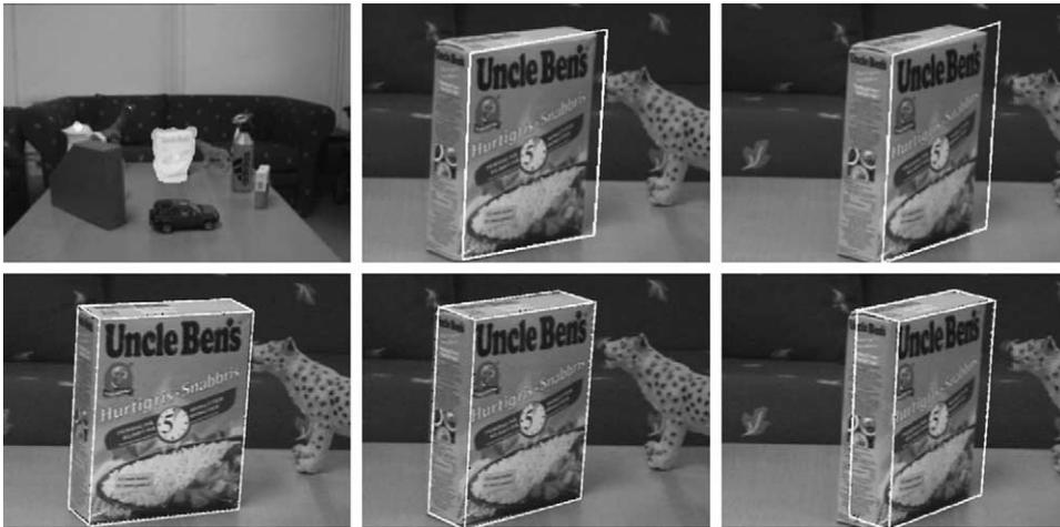
Fig. 13. From object hypotheses (upper left) the orientation of an object is estimated (upper middle/upper right). Pose estimates after three iterations for orientations  $20^\circ$ ,  $40^\circ$  and  $60^\circ$  (lower).
