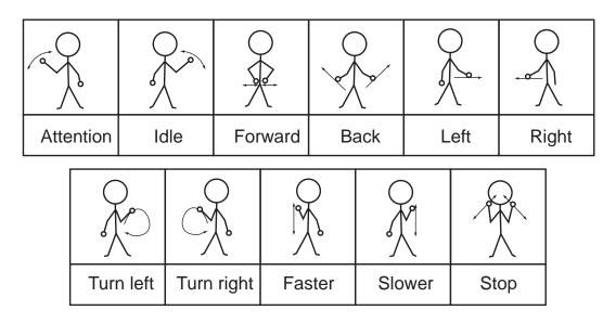
Figure 1: Example gestures for simple robot interaction
