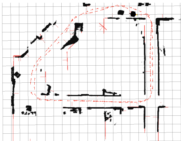
Fig. 11. A top-down visualization of a map produced from our low-clutter office environment. Many planar features are visible, including some that have been measured only by the 2D laser scanner. Planar features are visible by the red convex hulls, and red normal vectors. The small red arrows on the ground plane show the robot's trajectory. The small red arrows on the ground plane show the robot's trajectory. The point clouds used to extract these measurements are shown in white, and have been rendered in the map coordinate frame by making use of the optimized poses from which they were taken.
