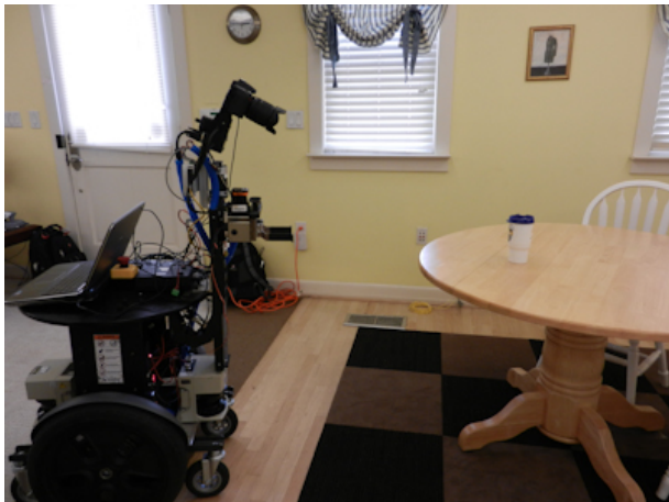
Fig. 5. The robot platform used in this work. Point cloud data is collected with the Asus Xtion Pro camera, and laser scan data is collected with the Hokuyo UTM-30. Both of these sensors are placed on the gripper near the middle of the robot. The Asus camera is mounted upside-down for more rigid and repeatable attachment.
