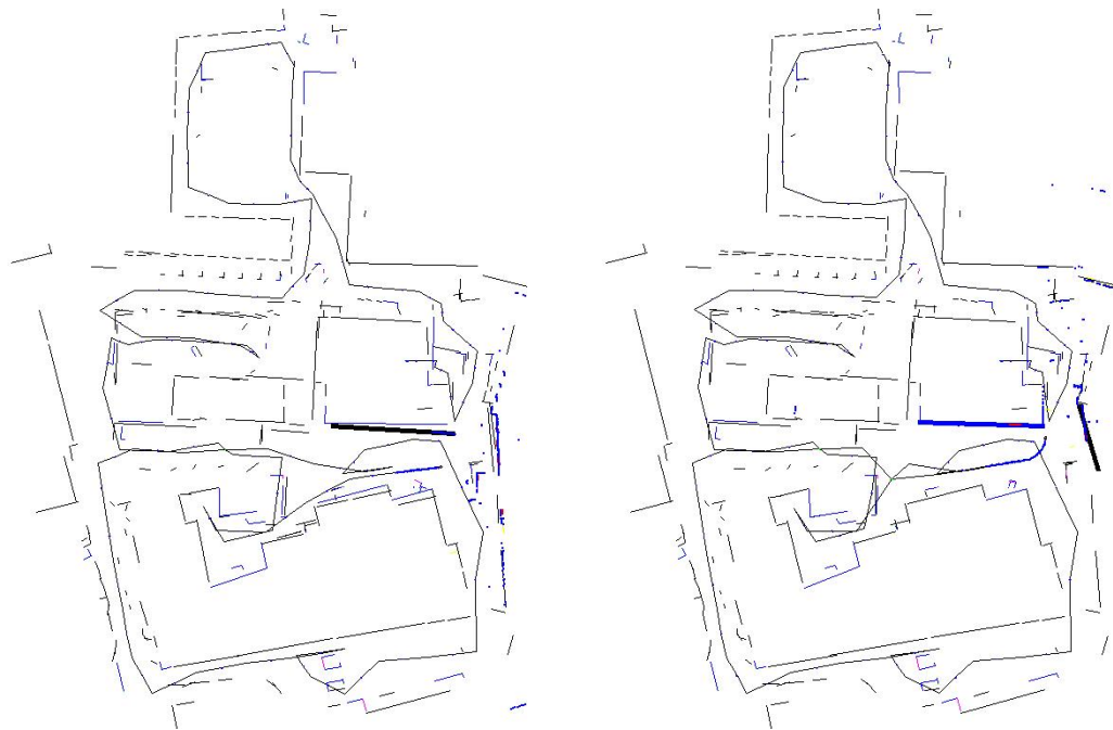
Figure 7: Here we show the third data set closing the second loop. We see the graph just as the loop is detected, left and just after the loop closing is performed, right.
