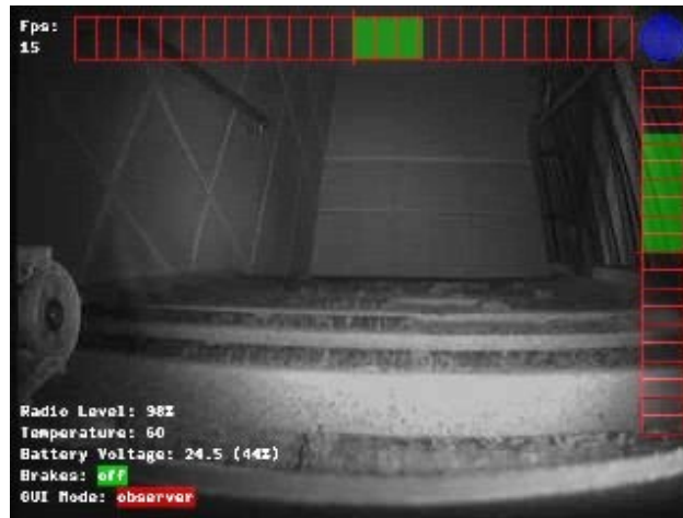
Fig. 6. The screen shown with video, speed information and telemetry data
