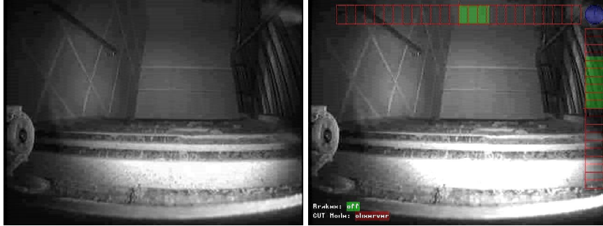
Fig. 5. The screen shown with video only information and with velocity information
