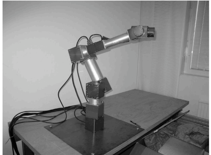
Fig. 1 The manipulator used for teleoperation studies
