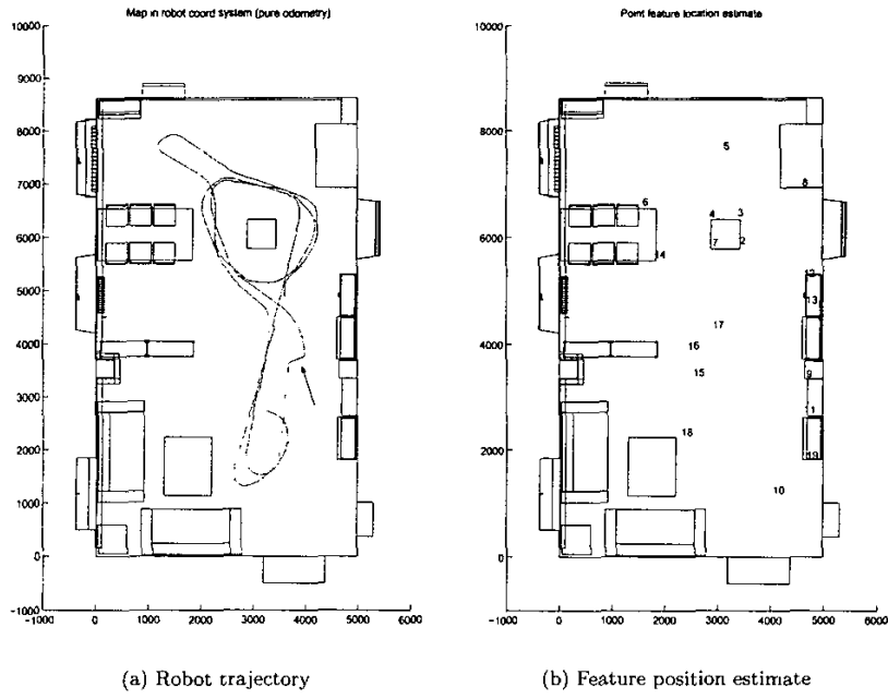
Figure 3: Trajectory of the robot in the living room and landmarks position estimate of the second experimental test.
