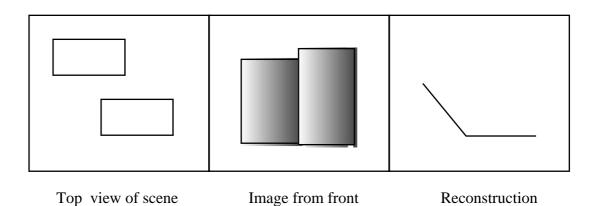
Figure 6. An example scene where an occlusion is present when view from the front. The left view shows the scene when viewed from the top. The middle view corresponds to the image. The right view to the reconstruction which is obtained when there is no
