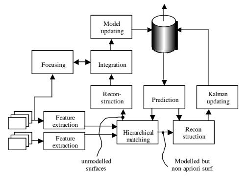
Figure 5. Block diagram for the cooperative stereo system.
