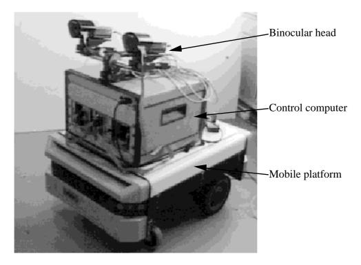
Figure 1. The AUC demonstrator system (ARVID).
