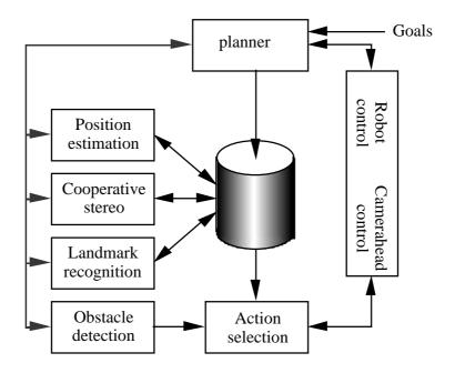
Figure 2. The vision sub-systems and their relation to the navigation system.
