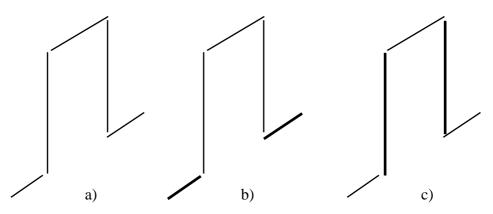
Figure 8. Outline of methods for recognition of landmarks (doorways). In figure a) line segments for the doorway are represented. In figure b) the segments used for detection of colinearity are shown. In figure c) the parallel segments from the landmark are shown.
