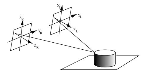
Figure 10. Geometry for a binocular set-up.
