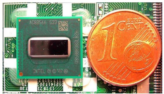
32-bit, Hyper-threading, low-power, inorder processors
