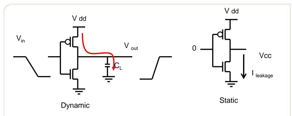
$$P_{tot} = P_{dyn} + P_{sta} = C_L V_{dd}^2 f + V_{dd} I_{leak}$$
