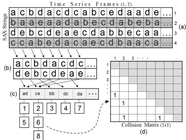
**Figure 2.** (a,b) For each iteration of random projection, a subset of string positions are selected (here, positions one and three). (c) The selected symbols are hashed, and (d) equivalent projections are tallied in a collision matrix.
