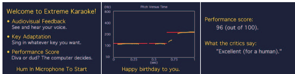
Figure 3: Screen shots from the multimedia Karaoke machine with voice-driven key selection, audiovisual feedback, and performance scoring. From left to right: splash screen; singing “happy birthday”; machine evaluation.
